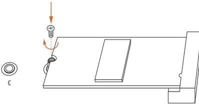
Tighten the screw with a screwdriver to secure the module into place. Please do not overtighten the screw as this might damage the module. Skip Step 6 if your M.2 SSD module is Type 2280.
